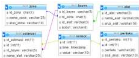
Figure 4.7 Design database estimation system of the household behavior
