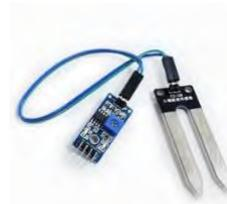
Gambar 2. Sensor Kelembaban Tanah
